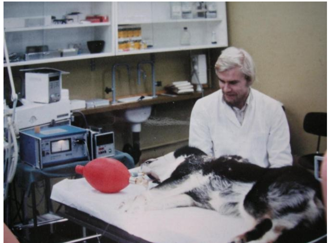
Pasi Talonen testing the phrenic nerve stimulator prototype with a dog in 1979.
